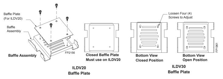
**NOTE:** Make sure the correct baffle plate is used.
